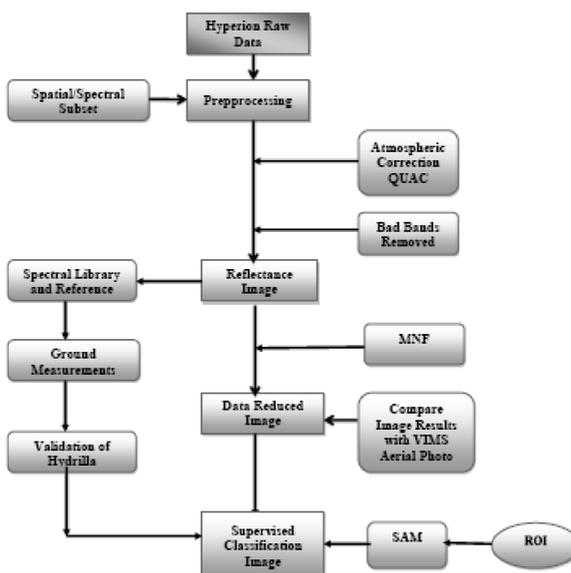
Figure 10: Flow Process Diagram for Image Preprocessing and Validation
